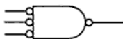
Fig. 4.8. Symbol for 3-input AND gate using negative logic assignment. (Functions as positive OR)
