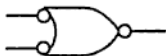
Fig. 4.12. Symbol for OR gate using negative logic. (Functions as an AND gate)
