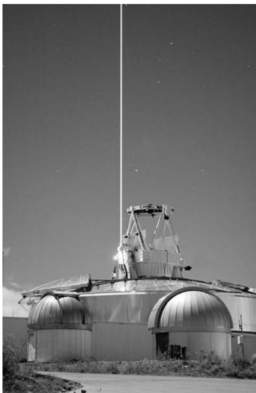
Figure 14.7 The 3.5-m telescope facility at the Starfire Optical Range in New Mexico with a 589-nm beam propagating to the mesosphere to produce a sodium guide star. (Photo courtesy of J. M. Telle.)
