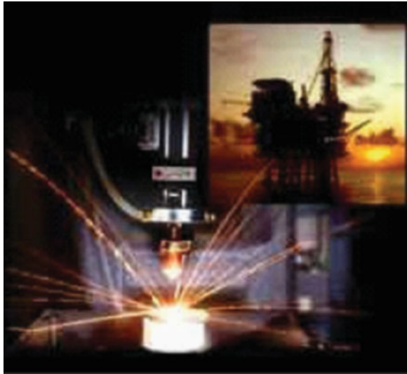
Fig. 19.7 Drilling through a piece of rock using laser. (Adapted from Ref. http://www.ne.anl.gov/facilities/lal/laser_drilling.html )
