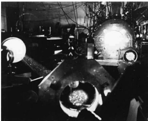
Fig. 16.3 A beam of infrared light from a Nd:glass laser after passing through a 10-cm aperture potassium dihydrogen phosphate (KDP) crystal (as left) is halved in wavelength (and hence doubled in frequency), emerges as green light at 5320 \text{ \AA} , and is reflected by the mirror at the foreground into the target chamber at far right. The 12.8-mm-thick KDP crystals have yielded doubling efficiencies greater than 60%. The output power was 0.5 TW ( = 0.5 \times 10^{12} \text{ W} ), one of the highest powers in the visible region of the spectrum. (Photograph courtesy: Thomas A. Leonard, KMS Fusion, Inc.)
