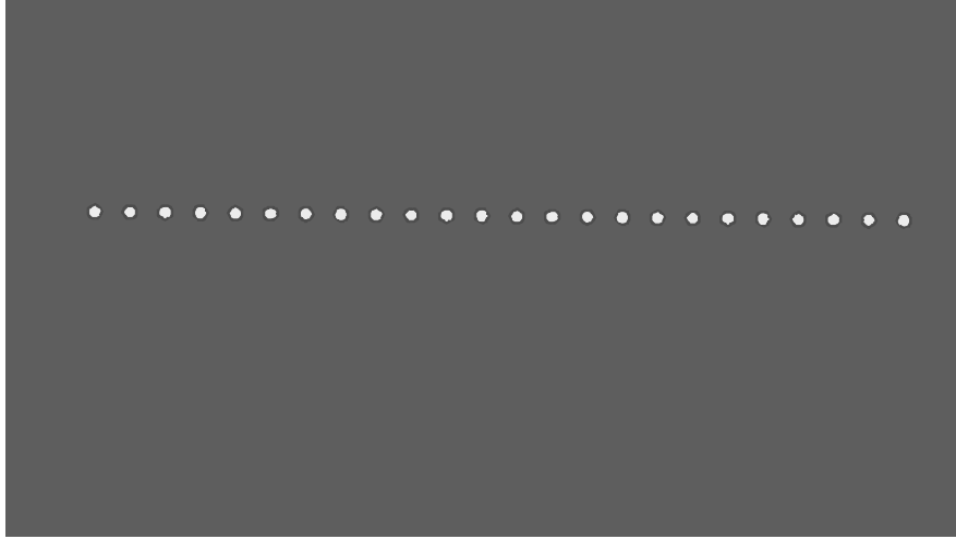
Fig. 22.30 Schematic of the intensity variation as seen from the top (or side) of an elliptic core fiber when a circularly polarized beam is incident on it. The actual photograph from an experiment by Andrew Corporation is given in Ref. 22.13.
