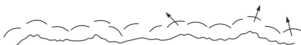
Fig. 12.8 Diffuse reflection of a plane wavefront from a rough surface. It is evident that one does not have a well-defined reflected beam.
