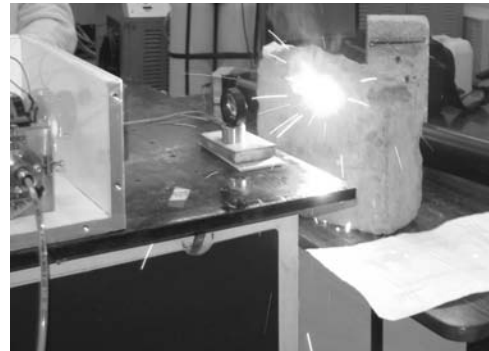
Fig. 40 Laser Drilling in Concrete at RRCAT using 1 kW Nd:YAG Laser. [Photograph courtesy: Dr. Brahma Nand Upadhyay, Raja Ramanna Centre for Advanced Technology, Indore.]
