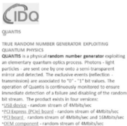
Fig. 2.21 A commercial product generating random numbers exploiting quantum physics; adapted from http://www.idquantique.com/component/content/article?id=9
