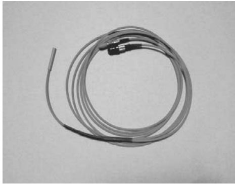
Fig. 28.21 Typical cabled probe used for displacement measurement; photpgraph courtesy: Dr Tarun Gangopadhyay, CSIR-CGCRI, Kolkata.
