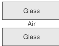
Fig. 15.3 Thin film of air formed between two glass plates.
