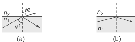
Fig. 28.4 (a) For a ray incident on a rarer medium ( n_2 < n_1 ), the angle of refraction is greater than the angle of incidence, (b) if the angle of incidence is greater than critical angle, it will undergo total internal reflection.
