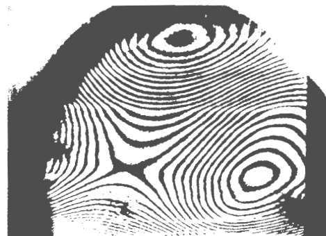
Fig. 15.28 A typical fringe pattern produced by an airfilm formed between two glass surfaces (which are not optically flat) and placed in contact with each other. Whenever the thickness of the airfilm is m\lambda/2 , we obtain a dark fringe and when the thickness is (m + \frac{1}{2})\lambda/2 , we obtain a bright fringe. Each fringe describes a focus of equal thickness of the film. [Photograph courtesy: Prof. R.S. Sirohi].
