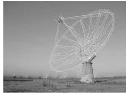
Fig. 2 Fully steerable 45 m paraboloidal dishes of the Giant Metrewave Radio Telescope (GMRT) in Pune, India. The GMRT consists of 30 dishes of 45 m diameter with 14 antennas in the Central Array. [Photograph courtesy: Professor Govind Swarup, GMRT, Pune].
