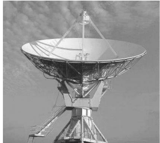
Fig. 3.7 A paraboloidal satellite dish. [Photograph courtesy: McGraw-Hill Digital Access Library. A color photograph of the above figure appears as Fig. 1 in the prelim pages].
