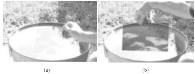
Fig. 22.12 If the sunlight is incident on the water surface at an angle close to the Brewster angle, then the reflected light will be almost polarized. (a) If the polaroid allows the (almost polarized) reflected beam to pass through, we see the glare from water surface. (b) The glare can be blocked by using a vertical polarizer and one can see the inside of the water. Figure adapted from the website http://polarization.com/water/water.html created by Dr J Alcoz; used with permission of Dr. Alcoz. A color photo appears as Fig. 29 in the prelim pages.
