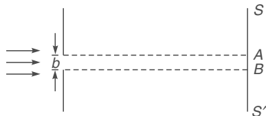
Fig. 18.1 If a plane wave is incident on an aperture then according to geometrical optics a sharp shadow will be cast in the region AB of the screen.
