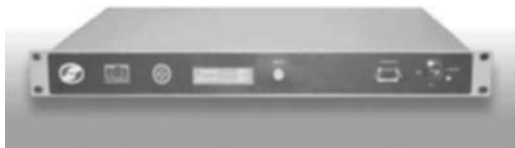
Fig. 27.10 An erbium doped optical fiber amplifier for telecommunication application developed jointly by CGCRI, Kolkata and NeST, Cochin. The main characteristics are: 32 wavelengths can be simultaneously amplified in the wavelength region from 1532 nm to 1565 nm. The input power (of each channel) can be between -4 dBm ( \approx 0.4 mW) to +3 dBm ( \approx 2 mW) and the output power is always 18 dBm ( \approx 63 mW) with a gain flatness of \pm 0.5 dB [Photo courtesy Dr. Shyamal Bhadra of CGCRI and Dr. Suresh Nair of NeST]; see also Fig. 38 in the prelim page.
