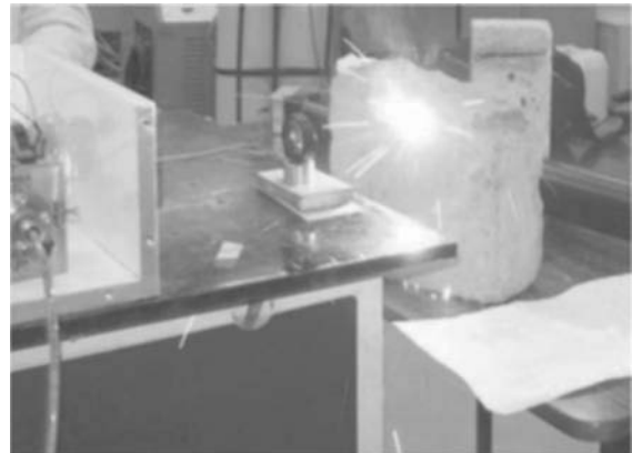
Fig. 18.19 A focussed laser beam drilling through concrete. Photograph courtesy: Dr. Brahma Nand Upadhyay, RRCAT, Indore. A colour photograph appears as Fig. 40 in prelim pages.
