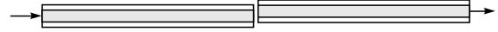
Fig. 30.5 A transverse alignment between two fibers would result in a loss of the optical beam.
