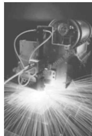
Fig. 27.13 A 2 kW fiber laser mounted to a robotic system cutting mild steel. [Photograph courtesy: McGraw-Hill Digital Access Library.]
