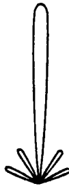
Fig. 6.6 Polar diagram of the array of Fig. 6.4, with a metal reflector added
