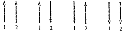
Figure 1.5 The four different states of a system of two elements numbered 1 and 2, where each element can have two conditions. The element is a magnet which can be in condition \uparrow or condition \downarrow .
