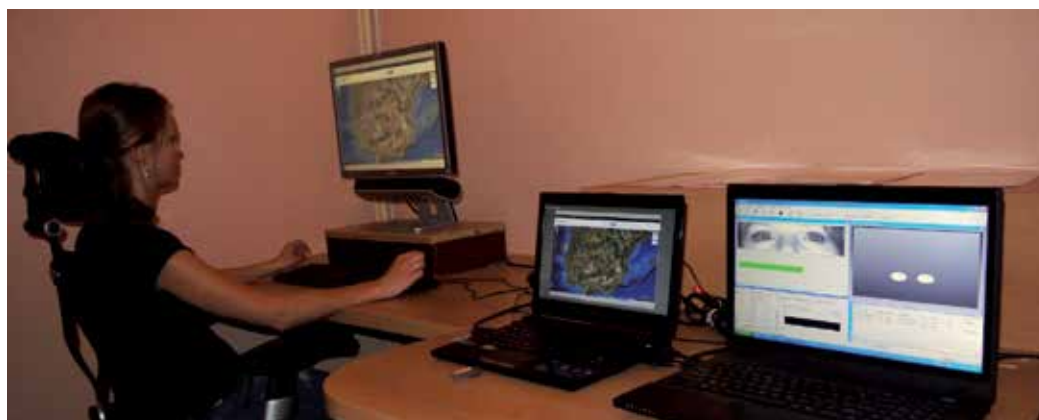
Figure 2. Laboratory setup with static remote SMI RED 250 eye-tracker at Department of Geoinformatics, Palacký University in Olomouc.
